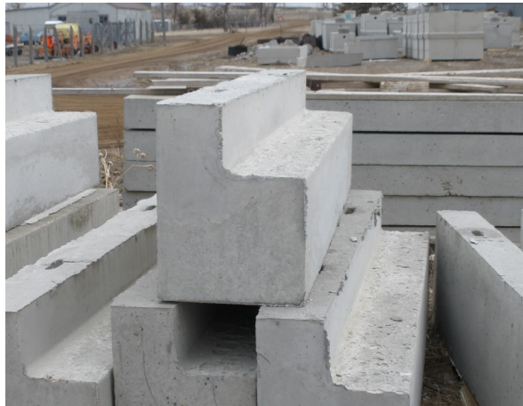
Cattle Guard Foundation Buttress in the precast yard.
